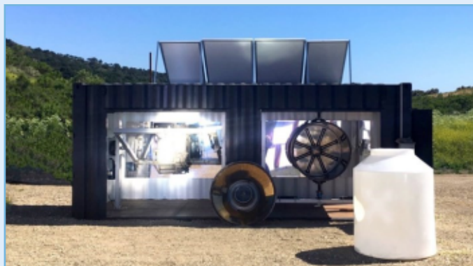
A solar rotational molding system with a sample rain catchment tank. Source: Light Manufacturing.
