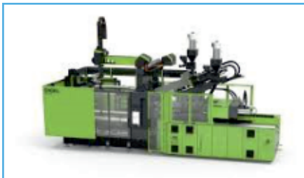
Fig 01: The insert 100's process optimization for overmoulding complex structures makes it easier to functionalize parts. Image: ENGEL
