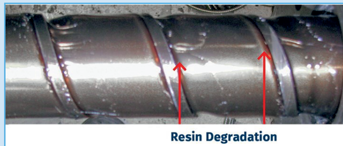
FIG 2 Degraded resin due to small flight radii because of Moffatt eddies.
