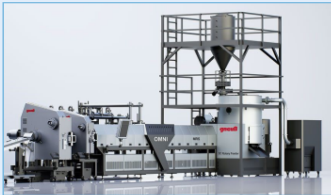
Fig.1: OMNI 200 Recycling System with 3C Rotary Feeder, MRS extruder, water ring pump vacuum system, twin RSFgenius screen changers and pelletizing line.
