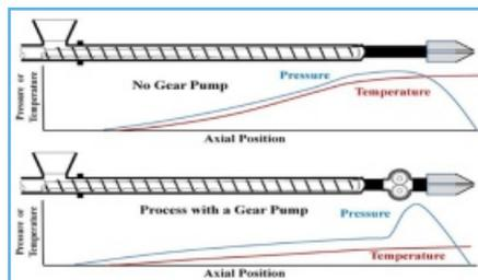
A gear pump positioned between an extruder and downstream equipment can improve the performance of a line. The advantages include the mitigation of pressure surges and as a result flow surges from the extruder; plus a decrease in the discharge temperature by generating part of the pressure required for the die by the pump, which reduces resin consumption and enables rate increases.
