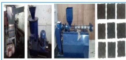
Indigenous equipment called single screw extruder developed for mechanical recycling through melt-mixing of waste thermoplastic polymers and inorganic particulate fillers can help manufacture and characterize polymer composites that can be molded to the required shape for making paver blocks, tiles, and bricks.
