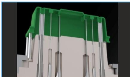
A review of materials, treatments and coatings to help determine the proper pins for optimized plastic part ejection. The most frequently used component of a mold's ejection system is the ejector pin, which includes variations such as sleeves and blades. Part size,
