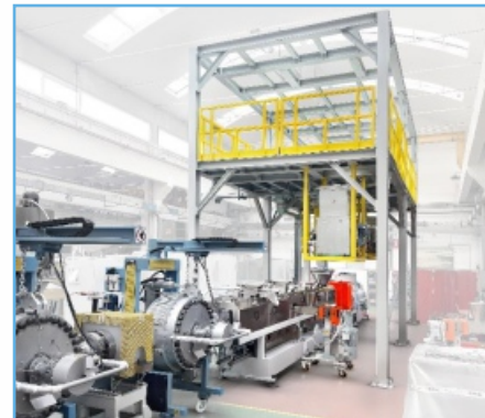
ICMA's line with MCM 110 extruder during installation
