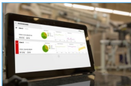
FIG 1 Intravis' IntraVisualizer remote monitoring software includes a dashboard and trend analysis with Estimated Time to Failure (ETF).
