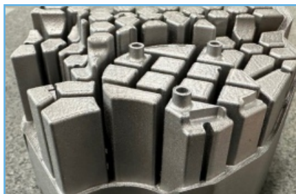
This core insert with conformal cooling channels was printed from HTC-45 powder.
