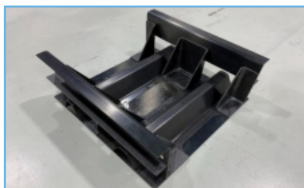
Thermally Welded Assembly of Aircraft Structural Demonstrator Applying This Technology
